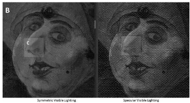
Figures 20 & 21: This is a comparison of symmetric and specular light scans. The images appear different because of differences in the ways in which incident light is reflected by the 3D texture of the image on the canvas.
